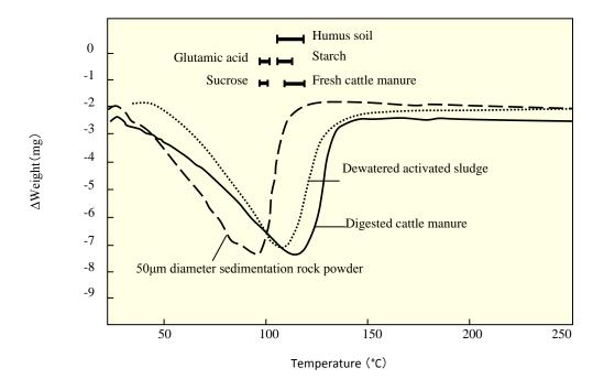
Fig. 7 Water retaining properties of some materials (TG measurements of some sludgy materials)  $N_2$  atmosphere, rate of heating: 10°Cmin<sup>-1</sup>
