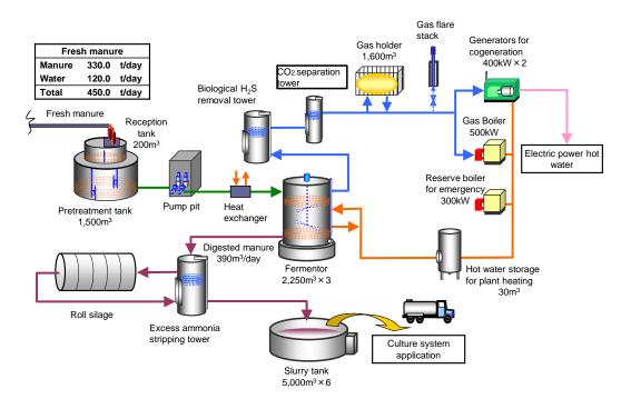
Fig. 1 A new biogas system with generation quartet functions
