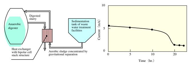
Fig. 8 A bio-fuel cell with a heat exchange structure
