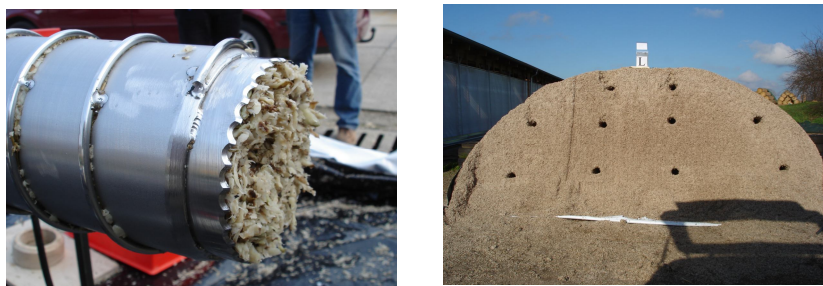
Figure 1. Filled drill (left) and positions of the cores at the transverse section of the tube (right)
